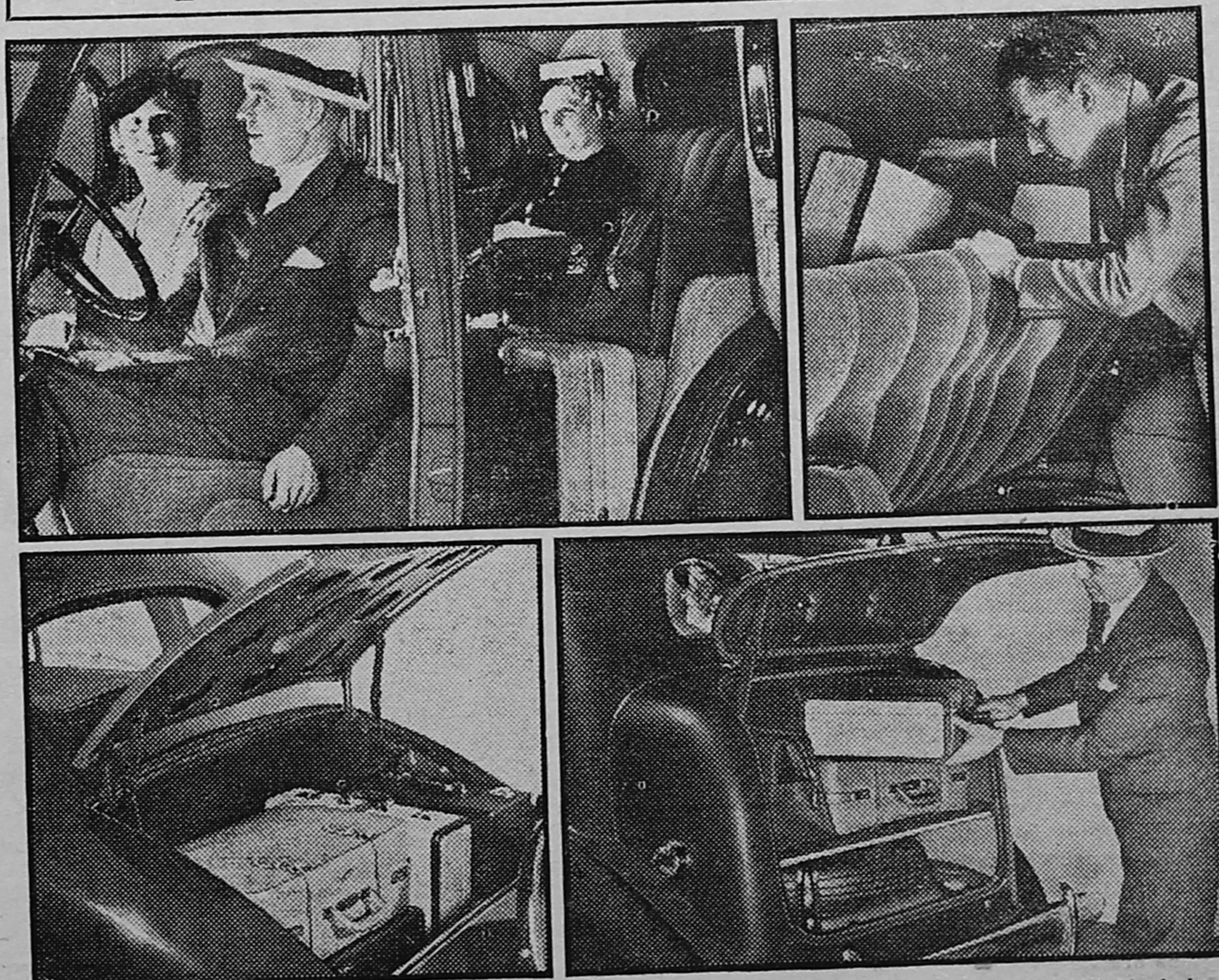
Comfort, pleasure, and safety on a tour depend largely on efficient loading of the luggage, and modern body designs have done much to ease the problem, as these views of Chevrolet models reveal. In the upper left view, the suitcases have been fitted snugly, the adjustable front seat having been moved forward to allow extra leeway, and the driver is now pushing back the seat to clamp the bags in place for the day. Upper right, the tourist is utilizing the baggage space back of the rear seat. The two lower pictures show the loading of a coupe compartment and a sedan trunk.
