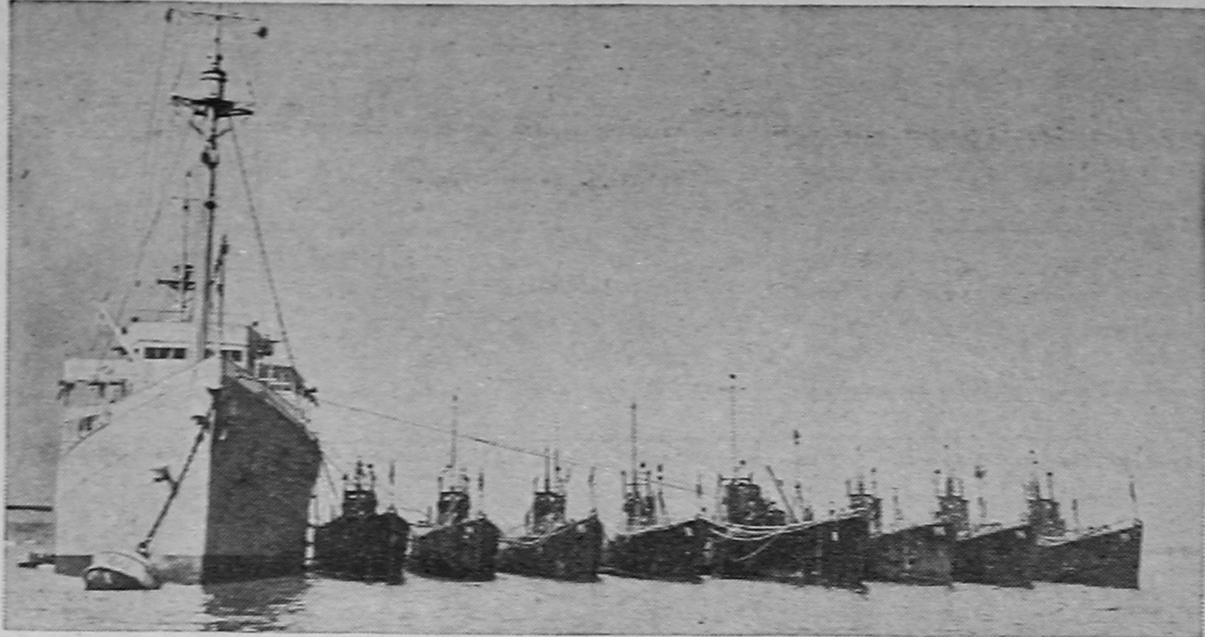
The U. S. S. Holland, navy submarine tender, pictured like a big mother as she serves as a buoy for her eight "chicks," submarines of the "P" series, the latest and most formidable undersea fighters in the world. The mother ship feeds her little ones fuel for themselves and supplies for their crews.
