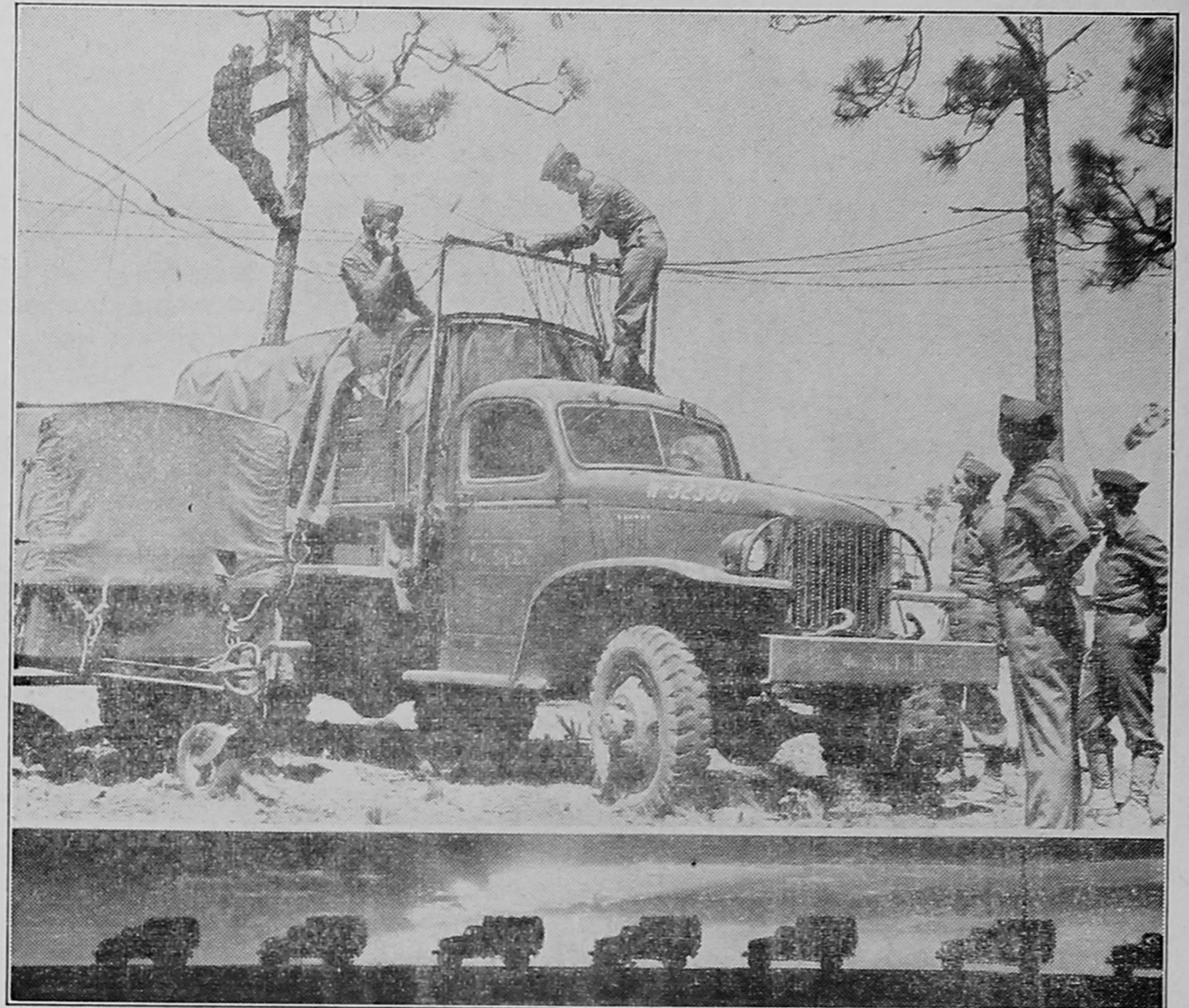
Uncle Sam's motorized force—the new army on wheels—is symbolized by the "dawn patrol" of Chevrolet 4 x 4 army trucks shown across the bottom of the photo. The Chevrolet four-wheel-drive army truck, above, carries a complete telephone switchboard. Within a few minutes after the Fourth Division's motorized units completed a 235-mile trek from Fort Benning, Ga., on a practice mass movement, Major-General Lloyd R. Fredendall could communicate with every part of the vast encampment. The Fourth, moving in three columns, each 45 miles long, made the trip in 10 hours as compared with nearly 10 days before motorization.
