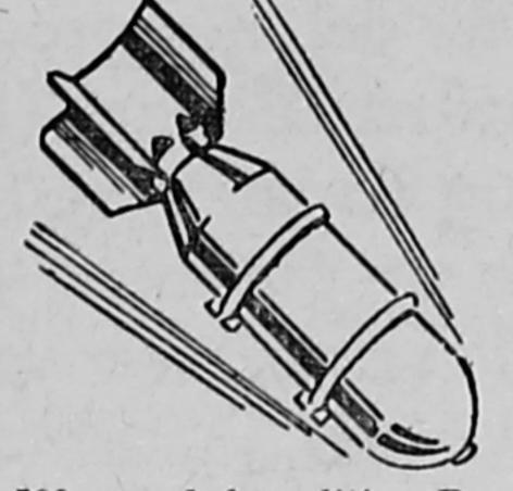
The 500-pound demolition Bomb is one of the lighter ones. Bands are attached to facilitate handling and the fins are not attached until the Bomb reaches the airfield, because bending would injure accuracy. They cost up to \$500. Your purchase of War Bonds through the Payroll Savings Plan will help provide Bombs for our airmen. Let's "Top that Ten Percent."
